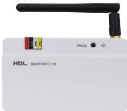
Figure 1. Wireless Mesh Gateway
