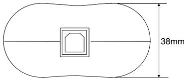
Figure 3. Dimensions - Side View
